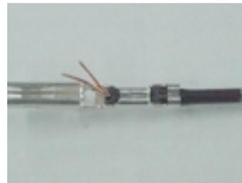
When the insulator enters crimp too much, the conductor barrel has broken strands before the lower dead point. So, the peak force drops drastically. This sudden change is clearly observed in the force curve.
