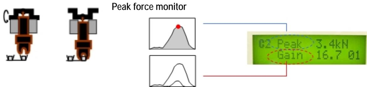
Normally original force level is too low. It is amplified to a suitable level. This amplification ratio is called as Gain. Normal gain is between 5 and 15
