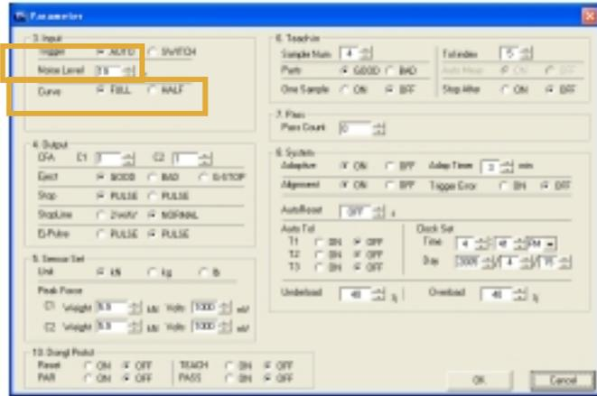
**Switch trigger** mode can select the automatic measurement mode. And it can select Full or Half curve.
