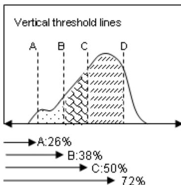
The whole x-axis 100% wide, and A to D lines are addressed by percentage (00%) in this coordination. Left edge is set as 0% and the right one is 100%. In this case you have to understand the force curve size before drawing A – D lines. For example, you have to monitor the force curve on ProMX before teach-in.
