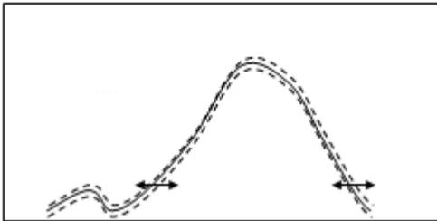
Force curves are likely to drift slightly, which affects measurement.
