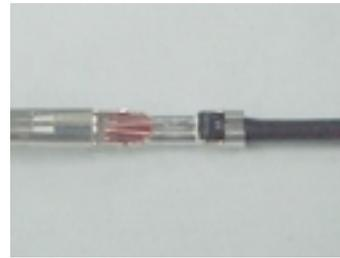
The peak level is normal but T1 or T2 area is abnormally high because conductor barrel has crimped the insulator together.
