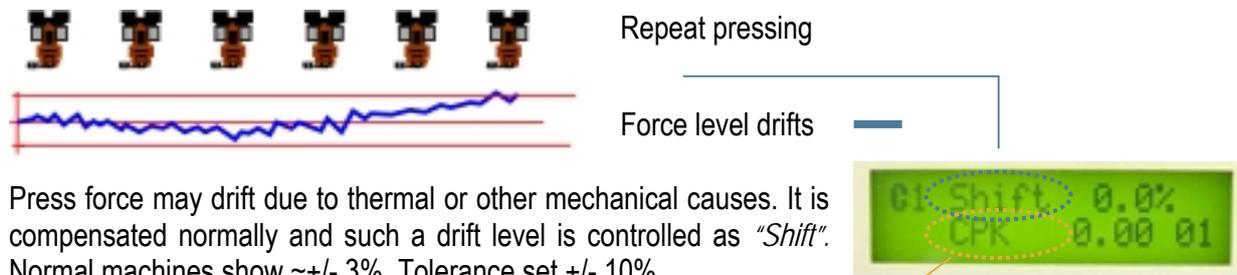
Press force may drift due to thermal or other mechanical causes. It is compensated normally and such a drift level is controlled as "Shift". Normal machines show  $\sim\pm 3\%$ . Tolerance set  $\pm 10\%$
