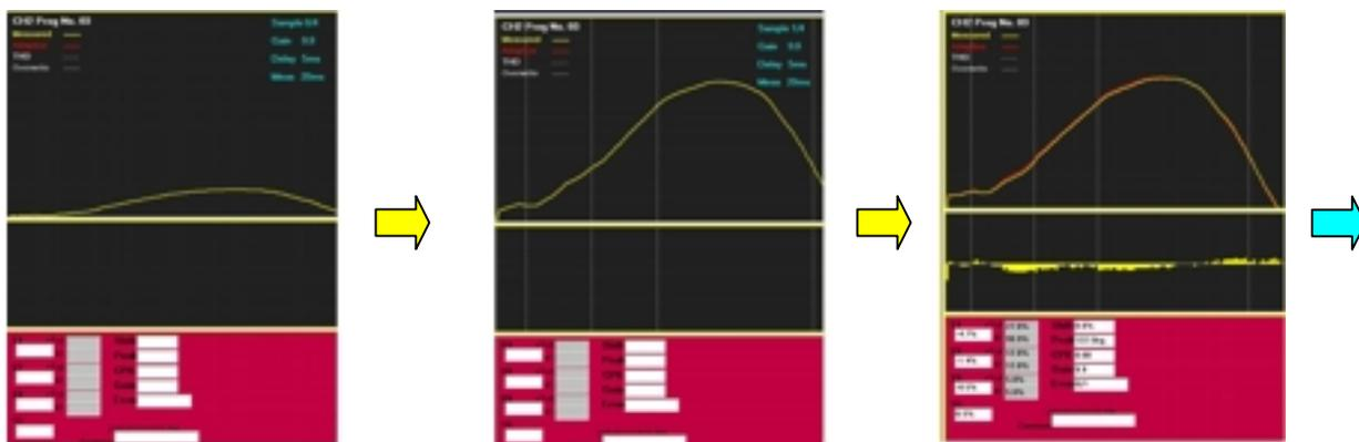
Start with raw force curve. Gain level 9.9, Trigger delay 5ms & Measure time 20ms
