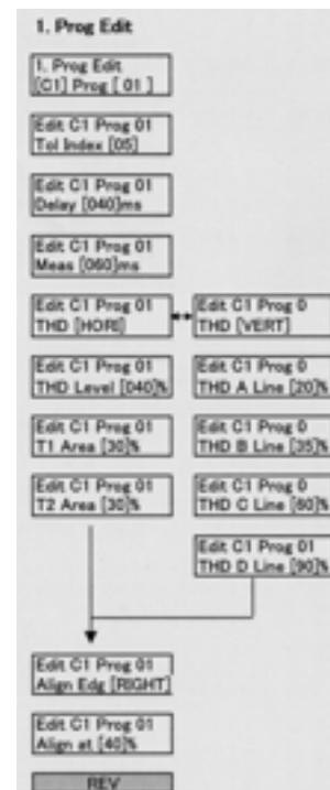
[Tolerance No]  All tolerance values are set in a tolerance number. There are total 20 patterns prepared in the tolerance table.
