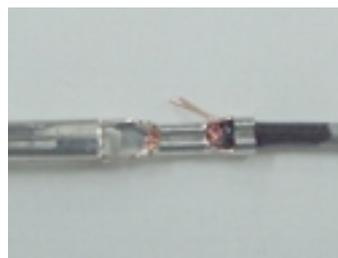
The error force curve drops for whole area normally. But, force shape does not distort so much. Similar curves appear at wire strands missing.
