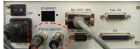
BNC cable connection to piezo force sensors
