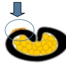
If the strands are coming out and crimped on the barrel, the total force doesn't change. Only crimp timing changes delicately. So, the start part of the force curve is higher a little. In the measurement area, T1 is high but T2 and T3 are normal.
