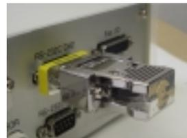
With the dongle key, you can program what function should be protected. For example, make RESET and TEACH as  OFF to prevent Pass and Parameters.
